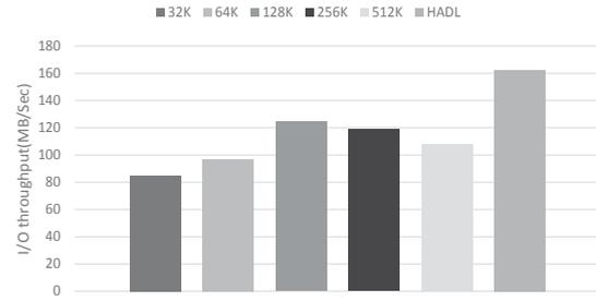
Fig. 14: Performance of LANL App2 with different layouts
