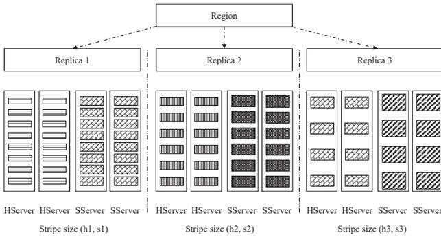
Fig. 7: The dynamic data layout scheme. Each region has three replicas, each with a different stripe size pair ( $h$  and  $s$ ) on HServers and SServers.
