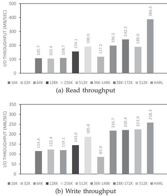
Fig. 12: I/O throughputs with non-uniform workloads
